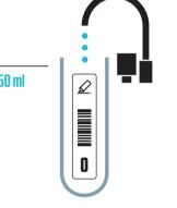
Fill to near the top of the tube with tap water immediately after opening the tap in the morning.
